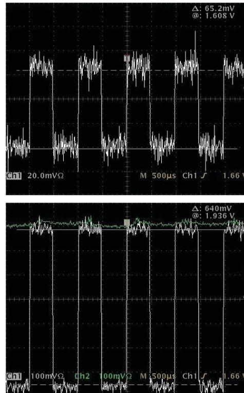
Fig. 14. Chopper amplifier I: (top) input voltage= $0.32\ \text{mV}$ ,  $k=100$ , square wave amplitude= $32.6\ \text{mV}$ ; (bottom) input voltage= $0.32\ \text{mV}$ ,  $k=1000$ , square wave amplitude= $320\ \text{mV}$
