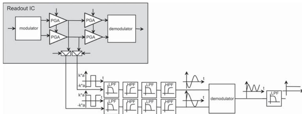
Fig. 19. The schematic view of the chopper circuit with selective AC amplifier, based on the designed IC
