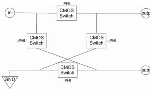
Fig. 2. Modulator architecture
