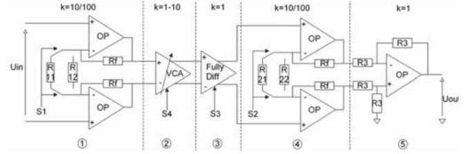
Fig. 11. The third AC amplifier circuit
