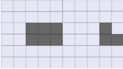
Fig. 4. Discretization grid allows representing heat sources as a set of squares
