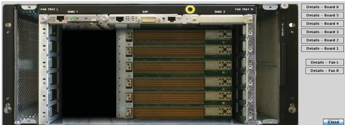
Fig. 2. A graphical software representation of the shelf front panel. The monitored shelf is empty. Buttons from the button section to the right, which refer to devices that are absent at a given moment, are inactive. This makes them slightly less distinguishable from their background.
