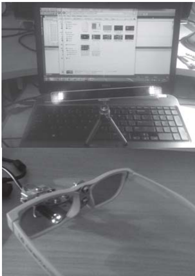
Fig. 6. Original project of optometric instrument (CinemaVision Movie Diagnostics) to perform measurement of stereoscopic movies.
